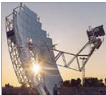
This solar dish-engine system is an electric generator that "burns" sunlight instead of gas or coal to produce electricity.
