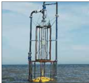
The SEADOG ocean-wave pump captures energy from ocean swells or waves to pump seawater to a land-based holding area or water tower, where the water can be returned to the ocean through hydroelectric turbines.
