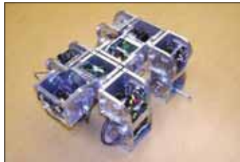
Modular robotic units self-assembled into this structure able to walk on four legs.
