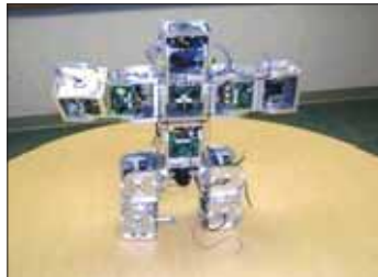
SuperBot modular robotic units self assemble into larger structures, such as this humanoid walker assembly, and micro-controllers. They can communicate with one another and even reshuffle themselves.
