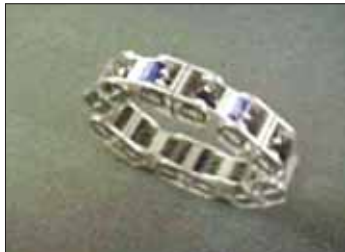
SuperBot modular robotic units assemble into a circular structure able to roll like a wheel.
