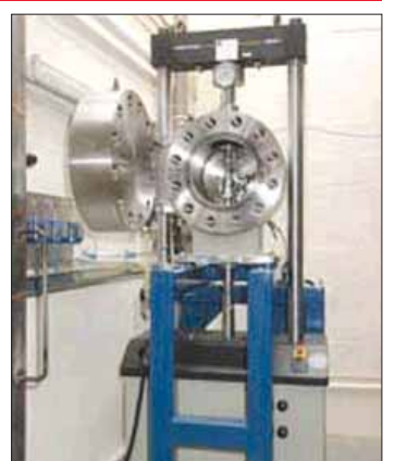
The current hydrogen vessel and testing machine has paved the way for TWI's new world leading version.
